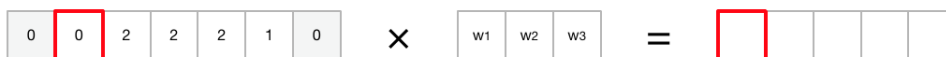
Abbildung 8: A 1D convolution where the filter values are represented as learnable weights
